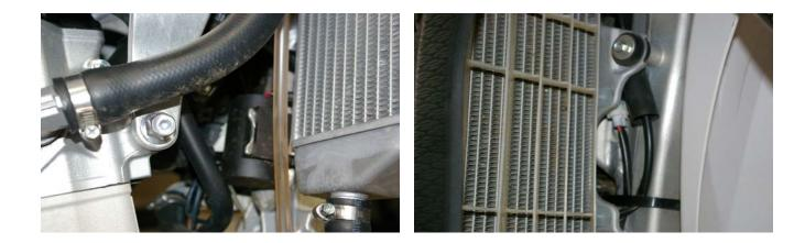
2. Unplug the factory connector and install the new harness with mating plugs to the factory connectors. Route the harness to the front of the bike to the steering neck area.
